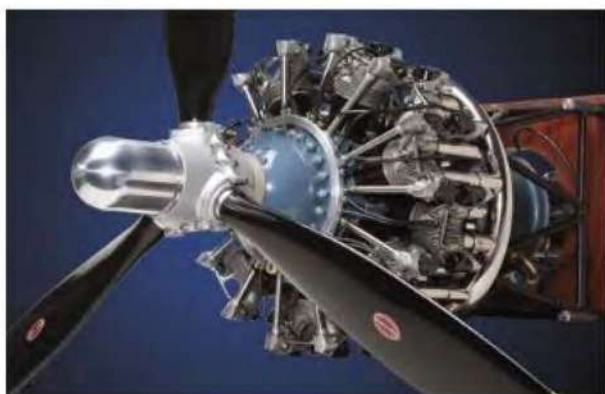
Radial - Multiple engines in a circle.
